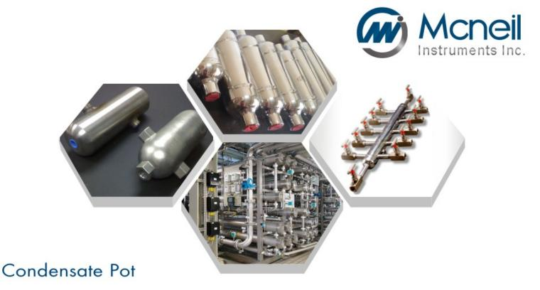
Condensate POT / Seal POT is a section of pipe (4inch in diameter) installed horizontally at the orifice flange union to provide a large -area surge surface for movement of the impulse line fluid with instrument element position change. It is used to reduce measurement error for hydrostatic head difference in the impulse lines.
